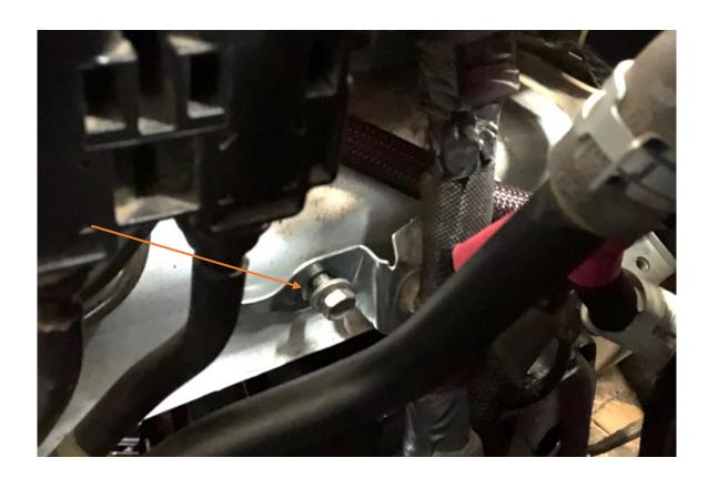
3. Set bracket back into open space so bracket holes line up with factory mounting points. Use product supplied hardware to secure top portion of bracket, and reuse factory hex head for the bottom of the bracket.
