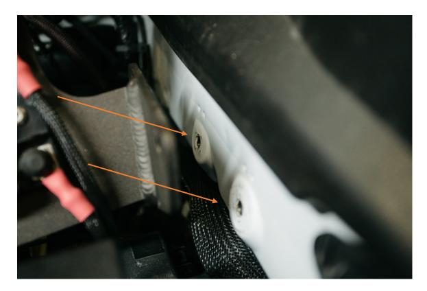
2. Follow the bracket leg down the engine compartment to find the hex head bolt near the right-hand side wheel well. This will mount the bottom portion of the bracket. Remove the bottom hex head bolt as seen in the photo. You will need to reuse this bolt.
