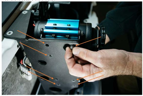
8. Connect or run all necessary wires to power the compressor. Then, reinstall the grill mount in reverse order to taking it off - placing the bottom end in first, then aligning the rest of the grill with the bumper and headlights. Reinstall the
