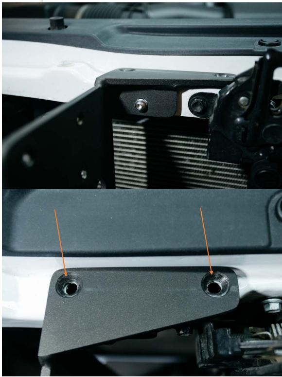
4. Insert 2 flat allen head bolts into the newly drilled holes, and finger tighten with flat washers and nylock nuts on the underside of the frame of the truck.
