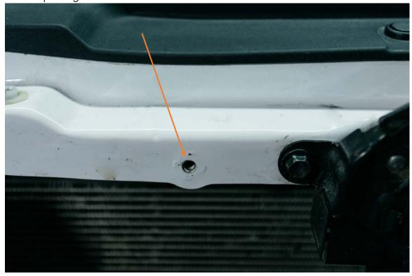
3. Set bracket up into the factory hole and insert a 6mm button head bolt to hold in place. You will need to drill the two top holes out. Drill holes with bracket secured in place.
