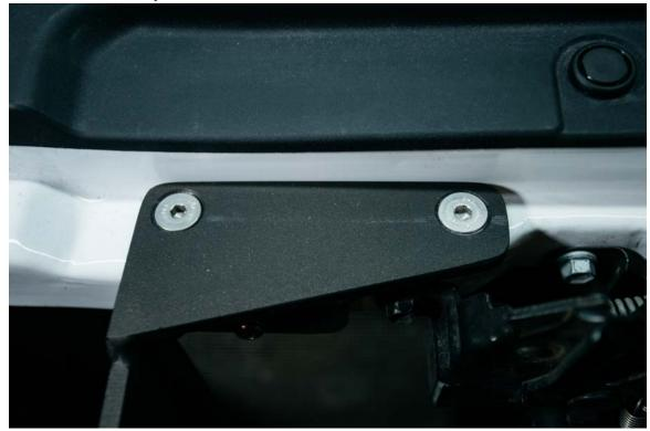
5. With the top bracket secure, ensure the holes align with the factory holes found on the bottom frame. Insert the back plate within the frame, align the holes, and insert the 8mm button head bolt with a lock washer and flat washer into the bracket - tightening through the back plate. Do this for both holes on
