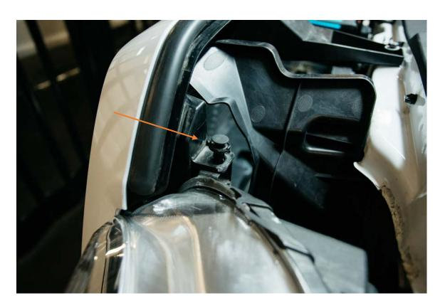
2. Find the factory threaded hole (6mm) just to the left (passenger side) of the hood-opening mechanism.
